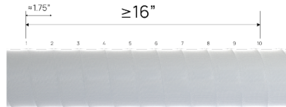
4" duct approximate wire helix pitch
